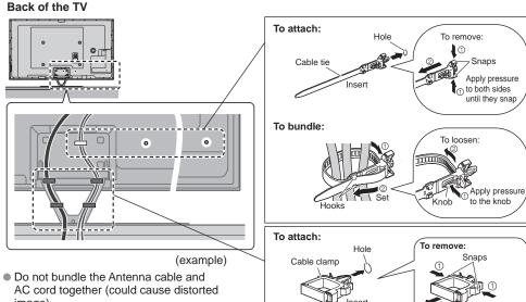
image).Fasten the cables with the Cable tie/ clamp as necessary.
