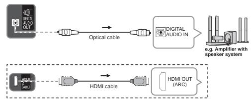
HDMI connection is available if connected audio equipment has ARC (Audio Return Channel) function.
